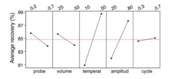
Fig. 2. Main effects plot of variables on the average relative recovery of phenolics. Probe: diameter of probe used; volume: volume of extracting liquid; temperature: extraction temperature; amplitude: amplitude of ultrasounds (percentage of maximum ultrasonic power); cycle: pulse of ultrasound in fractions of second.
