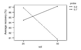
Fig. 3. Effects of interactions between extracting volume and ultrasonic probe over the average recovery phenolics.
